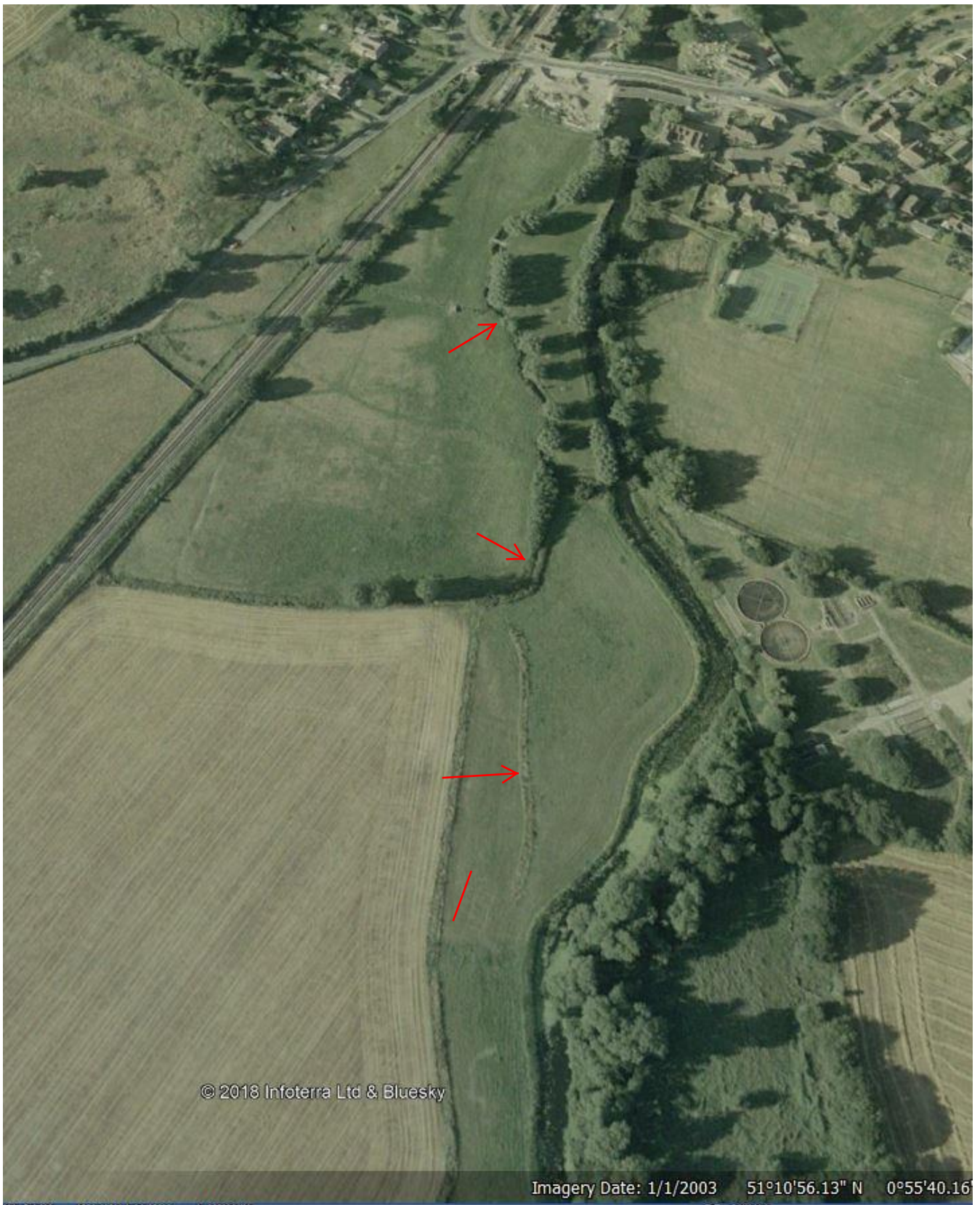
AP4. The 2003 aerial from Google Earth shows the site of Roman Industrial Building (red line) and the water leat running north and south with water flow strongest as it comes off the River Stour and a drop of 1m every 100m. Red arrows show course of the Roman leat (watercourse) to the north and the sea.
